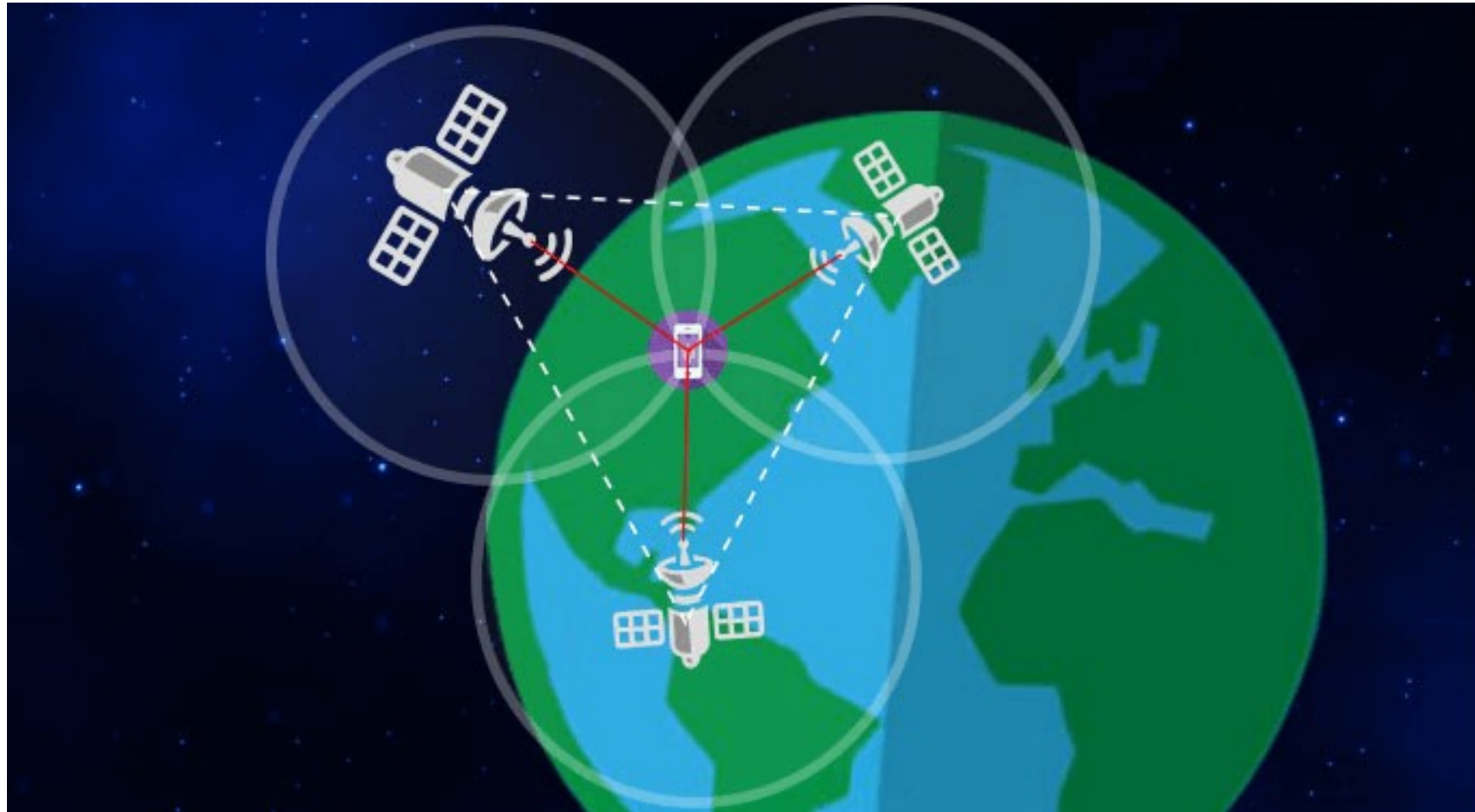
Fig: Trilateration Principle
